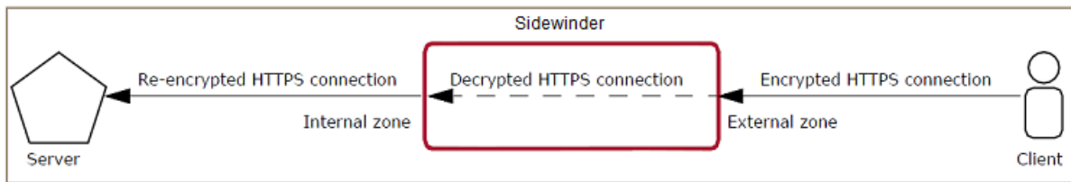
Figure 23: Inbound connection with decryption and re-encryption
