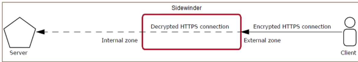
Figure 22: Inbound connection with decryption
