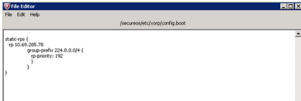
Figure 26-11 Bootstrap router parameters
