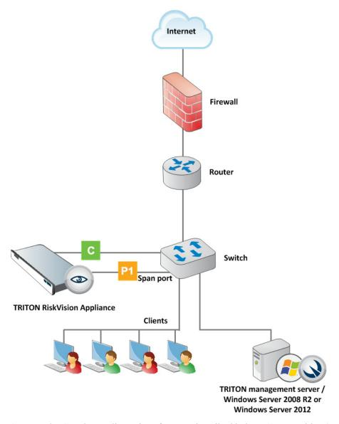
Connect the C and P appliance interfaces as described below. Cat 5E cables (or better) are required. Do not use crossover network cables.
