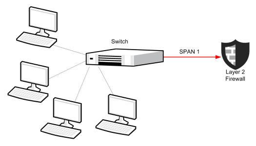
When you select Only Log Connection mode for the global Default Connection Termination, you can deploy Layer 2 Firewalls in Passive Firewall mode in an inline configuration.
