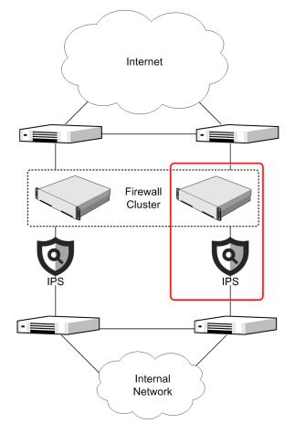
Redundant single inline IPS engines alongside a Firewall Cluster
