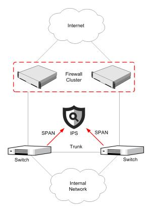
In a redundant disaster-recovery setup, Firewall Cluster nodes can be far apart. The IPS engines are not clustered in this configuration, but they have identical policies.
