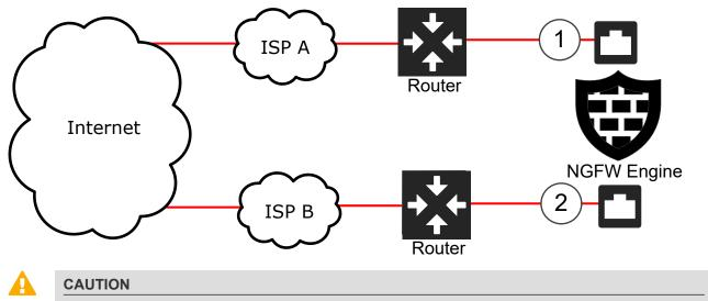
We do not recommend defining two or more IP addresses for a single physical interface. If two IP addresses are defined, the router behind the interface forwards the traffic to the different ISPs. This creates an additional single point of failure at the intermediate router, and the associated cabling and network cards.
