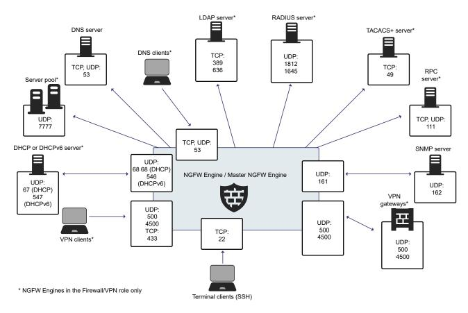
This table lists the default ports for NGFW Engines and Master NGFW Engines. Many of these ports can be changed. The names of corresponding default Service elements are also included for your reference.
