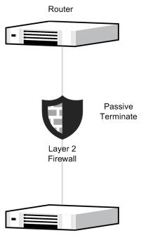
Passive Firewall: a Single Layer 2 Firewall in passive inline mode
