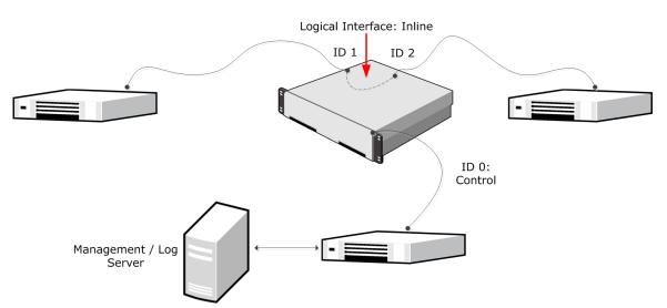
In this example, the IP address on Interface ID 0 is configured as the Control IP address for management connections. Interface ID 1 and Interface ID 2 are an inline interface pair that share the Logical Interface, called
