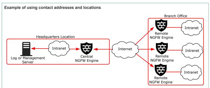
In this example scenario, a Management Server and a Log Server manage SMC components both at a company's headquarters and at three branch offices.
