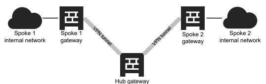
All traffic from the Spoke 1 internal network to the Spoke 2 internal network, and from the Spoke 2 internal network to the Spoke 1 internal network is sent through a VPN tunnel to the hub gateway. The hub gateway forwards the traffic through another VPN tunnel to its destination.
