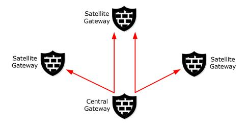
*VPN hub topology* routes site-to-site or mobile VPN connections to other sites through a central (hub) gateway using other site-to-site VPNs. The hub is usually a central gateway, but it can also be a satellite gateway.
