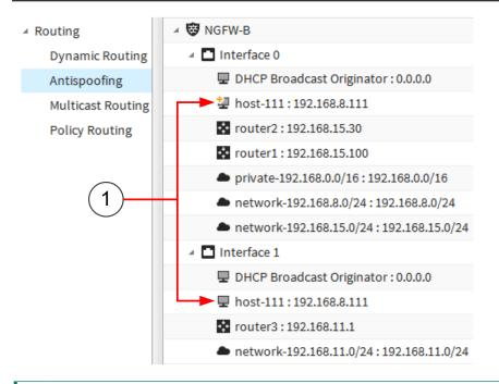
1 Both Interface 0 and Interface 1 are considered valid sources for host-111 (192.168.8.111) because the Host element is beneath both interfaces. The plus sign on the host on Interface 0 indicates that the host was manually added to the configuration. Traffic can originate from both Interface 0 and Interface 1.
