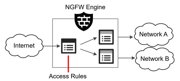
In the illustration, traffic is checked against the Access Rules, and allowed traffic is assigned a QoS Class. At the interfaces connected to the internal network, the QoS Policies limiting the bandwidth use are enforced as the traffic is sent onwards.
