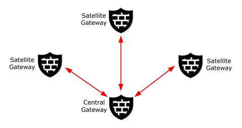
*Star topology* connects sites behind satellite gateways to the sites behind central gateways. No VPN tunnels are established between the satellite gateways.
