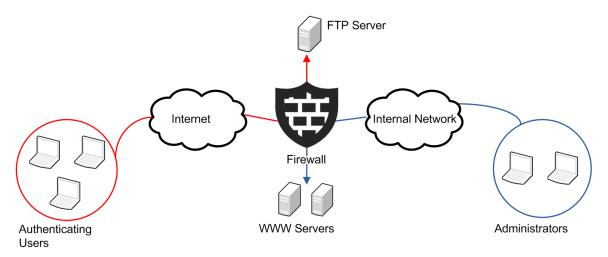
The WWW servers must be accessible to anyone from both internal and external networks. HTTP traffic is inspected against the Inspection rules, excluding the administrators' own PCs (on the right in the illustration) because they often test the servers for vulnerabilities. The FTP server is accessible to all users in the general office network, but only to certain external users (on the left) that authenticate using an external authentication server.
