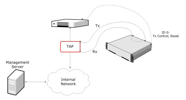
In this example, Interface ID 0 is a Normal Interface used for management connections, and sending TCP Reset responses. Interface ID 1 is a Capture Interface that listens to the received (Rx) packets from the network TAP. Interface ID 2 is a Capture Interface that listens to transmitted (Tx) packets from the network TAP. Interface IDs 1 and 2 share the Logical Interface, which combines the traffic from both physical interfaces so that it can be inspected as a complete traffic flow.
