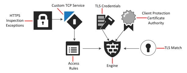
The TLS Credentials and the Client Protection Certificate Authority elements are specified in the properties of the engine that provides TLS Inspection. The engine uses the private key and certificate stored in the TLS Credentials to decrypt traffic to and from TLS servers in the protected network for inspection.
