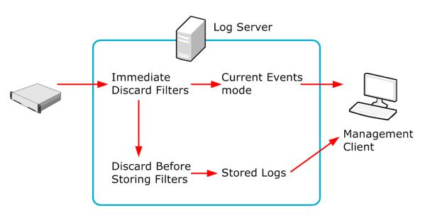
The engines send their logs to their configured Log Server. The Log Server either stores the log entries or just relays them to be viewed immediately in the Current Events mode in the Logs view. Some logs might be discarded through pruning before these operations. When you view logs, the information is fetched directly from the Log Servers. Some other tasks, such as processing data for statistical reports, are also partially carried out by the Log Server.
