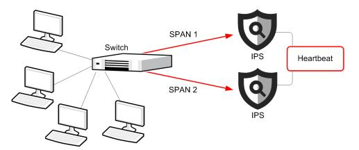
An IPS Cluster can be deployed alongside a Firewall Cluster. In this configuration, the IPS Cluster is in the same broadcast domain as the Firewall.
