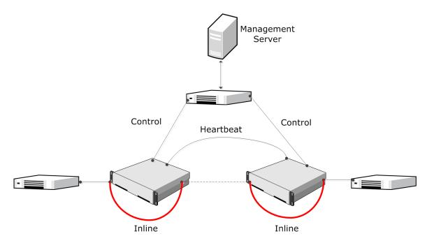
In this example, the IPS Cluster consists of two nodes. Interface ID 0 is a Normal Interface used for the heartbeat communication between the nodes. Interface ID 1 is a Normal Interface used for communication with the Management Server. Interface ID 2 and Interface ID 3 are an Inline Interface pair that share one Logical Interface, called Inline. Traffic enters each IPS node through Interface ID 2 and leaves through Interface ID 3.
