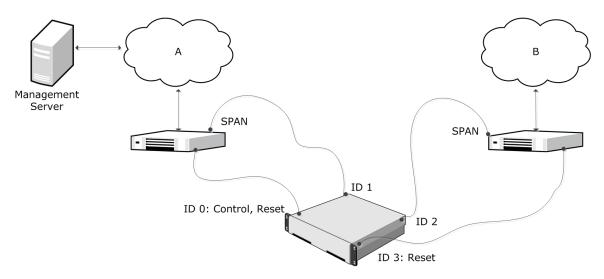
In this example, Interface ID 0 is a Normal Interface used for management connections, and sending TCP Reset responses for network segment A. Interface ID 1 is a Capture Interface for capturing network traffic from the network segment A switch for inspection. Interface ID 2 is a Capture Interface for capturing network traffic from the network segment B switch for inspection. Interface ID 3 is a Normal Interface used for sending TCP Reset responses for network segment B.
