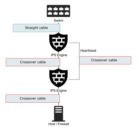
Correct cable types for Active/Standby Layer 2 Firewall Clusters
