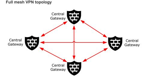
*Full-mesh topology* connects each site to every other site in the same VPN. All gateways are central gateways, which means that all gateways can establish tunnels with all other gateways in the VPN. The full mesh topology is formed between sites that must all be able to connect to any other site.
