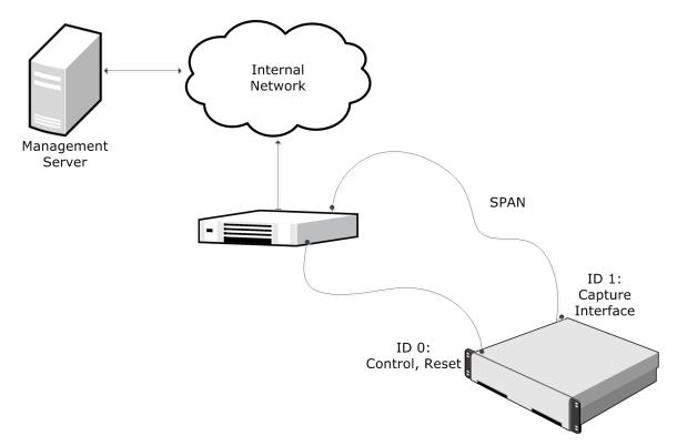
In this example, Interface ID 0 is a Normal Interface used for management connections and sending TCP Reset responses. Interface ID 1 is a Capture Interface used for capturing network traffic from the network switch for inspection.
