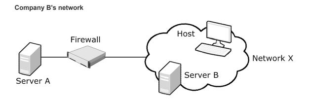
Server A provides services to users in network X, as well as to Server B. The administrators are interested in tracking how many of the users in network X actually use Server A. Server B also connects frequently to Server A, and generates a large amount of traffic.
