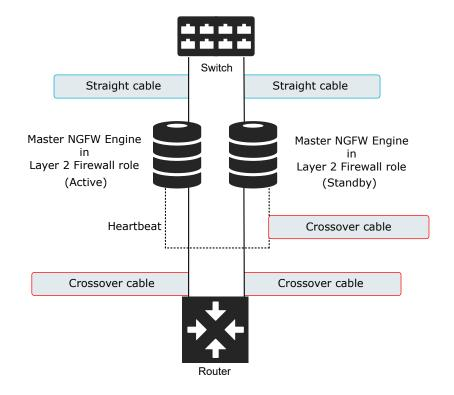
Correct cable types for Active/Standby Virtual Layer 2 Firewall Clusters
