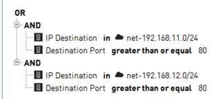
A filter has the **IP destination** and **Destination port** fields. ICMP traffic, for example, does not have the **Destination port** field. If ICMP traffic is matched with the example filter, the filtering results vary according to the selected Undefined value policy:
