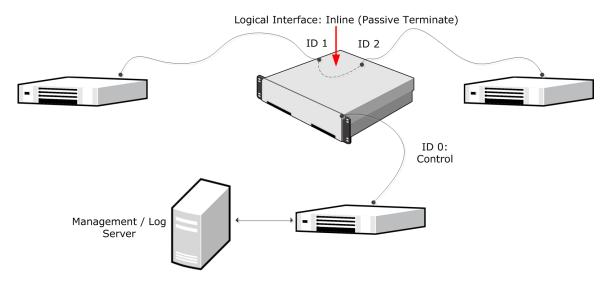
In this example, the IP address on Interface ID 0 is configured as the Control IP address for management connections. Interface ID 1 and Interface ID 2 are an inline interface pair that share the Logical Interface, called Inline (Passive Terminate). Traffic comes in through Interface ID 1 and leaves through Interface ID 2.
