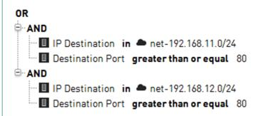
The illustration shows a Filter with several fields and operations. This Filter matches if the destination IP address is in the 192.168.11.0/24 network AND the destination port is 80 or greater OR if the destination IP address is in the 192.168.12.0/24 network AND the destination port is 80 or greater.
