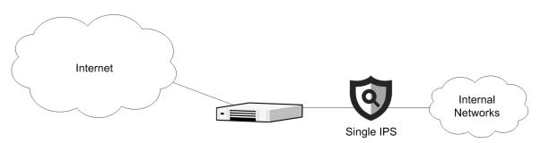
To inspect the low-volume traffic that the end users' Internet and VPN-bound communications generate, the company installs a Single IPS at the office. Because there are no local administrators and the traffic volumes are low, the logs are sent to the Munich Log Server. When the logs are sent to the Munich Log Server, it is quick and easy for the responsible administrators there to view and manage the data.
