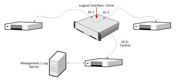
In this example, the IP address on Interface ID 0 is configured as the Control IP address for management connections. Interface ID 1 and Interface ID 2 are an Inline Interface pair that share the Logical Interface, called Inline. Traffic comes in through Interface ID 1. Any traffic that is allowed by the IPS engine leaves through Interface ID 2.
