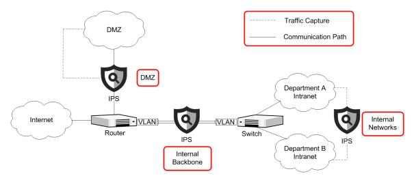
The illustration outlines common deployment scenarios for IPS engines in general internal networks and in DMZ networks. Layer 2 Firewalls can be used in similar scenarios. IPS engines and Layer 2 Firewalls are not
