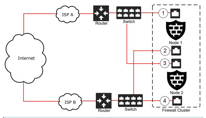
1 Interface 1 on Node 1 is used as the CVI for Internet traffic that is routed through ISP A.
