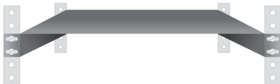
2. Place appliance on tray and secure to server rack using mounting screws on front of appliance.
