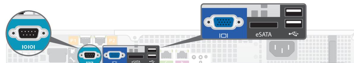
Connect a computer to serial port using null modem cable (provided). Or, connect a terminal server to serial port using a straight-through cable (not provided). *Serial port settings are: 9600 baud, 8 bits, no parity.*
