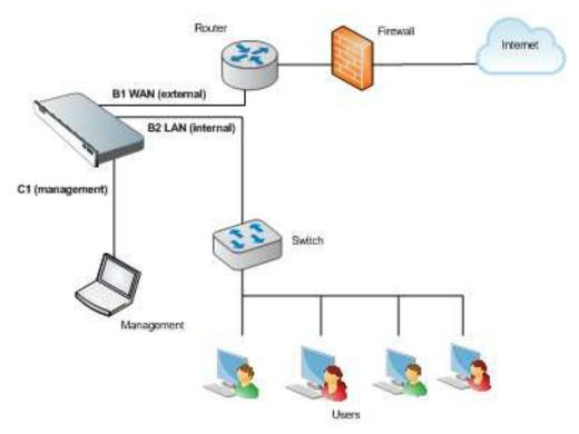
If your network includes a firewall, you need to ensure that destination TCP ports are open for connection to the cloud service. By default, the appliance is configured to use standard destination ports 80 and 443 for these connections.
