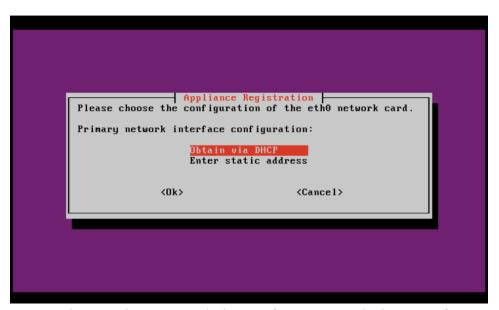
Forcepoint strongly recommends the use of DHCP. An IP in the range of 10.0.0.200-254 will be assigned to each Advanced Malware Detection On-Premises Engine on the private engine network. The Advanced Malware Detection On-Premises Engines will obtain IPs via DHCP from the Advanced Malware Detection On-Premises Manager over the engine network.
