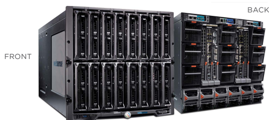
The Websense X10G blade server scales from 2 to 16 blades all within a 10U extensible chassis architecture.
