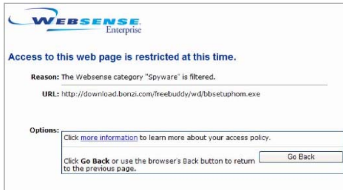
Figure 5. Security PG prevents employees from accessing sites that have been categorized as spyware Web sites.
