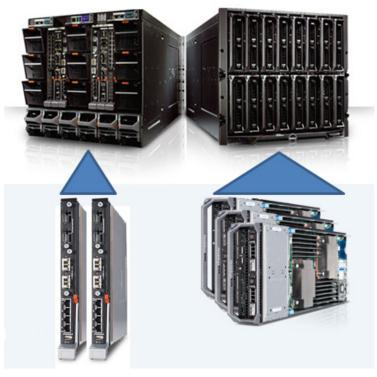
X-Series appliances come with two Dell PowerConnect M6220 switches. When used with the X10G<sup>TM</sup>, each switch supports two 10Gb SFP+ ports.
